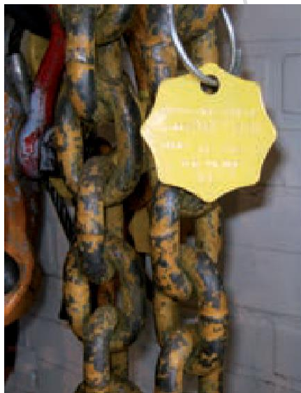
Different kinds of lifting equipment with colored inspection marks.
