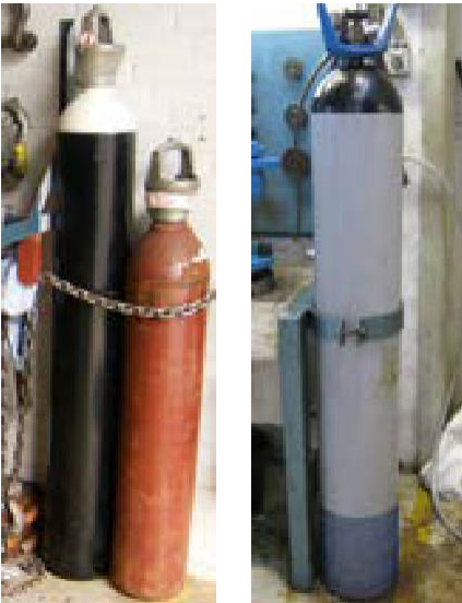
No risk of overturning. Securely fastened.
