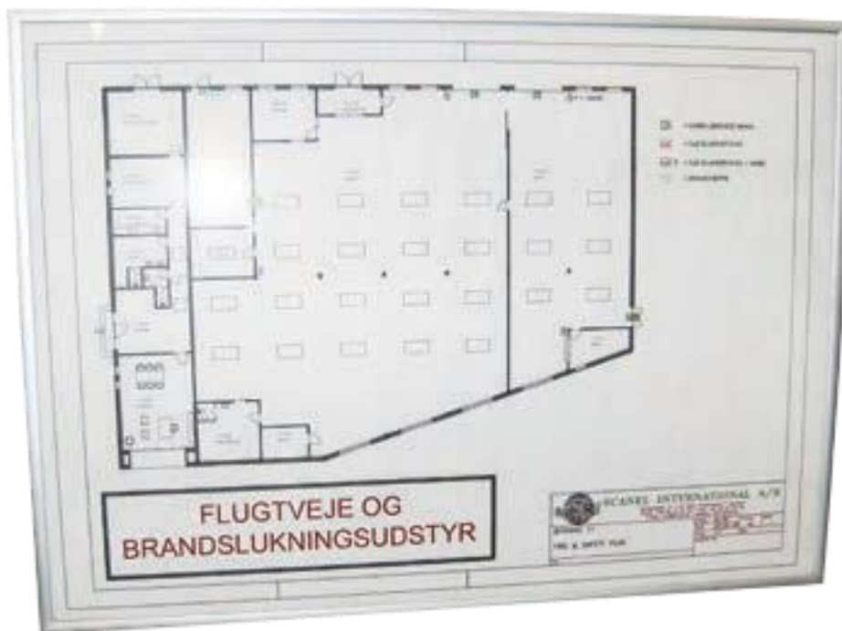
At all Scanel locations you will find these carts that describe the fire exits and the position of fire extinguishers of the specific location.
