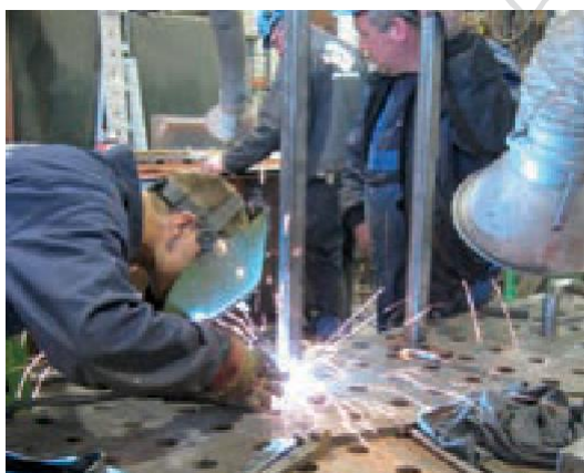
Local exhaust could be drawn even closer
