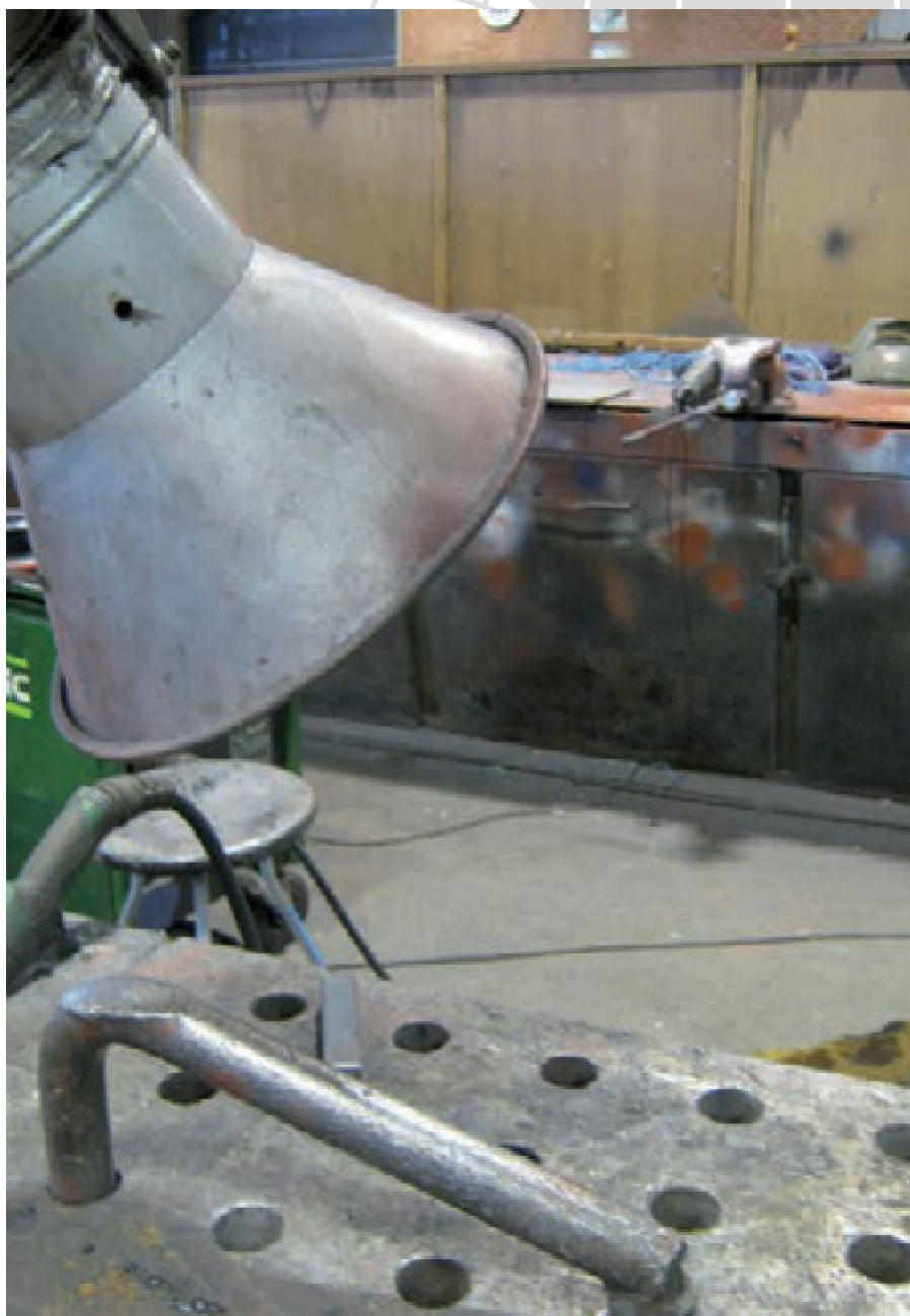
Local exhaust placed right over the working area.
