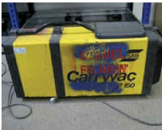
Movable exhaust for welding or other tasks that produce smoke or gasses.
