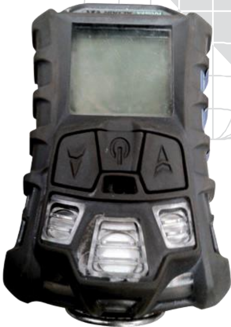
Gastester. An instrument for measuring the content of various gasses in the air.
